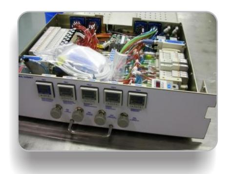
NEHP can design, fabricate, test and ship any type of process utility equipment or prefabricated assembly, for multiple industries, no matter what the intended purpose. Our skilled engineers are experienced in all of these fields. Shown here is a custom-designed, electro-pneumatic control module for a sophisticated semiconductor process tool. NEHP is the supplier of choice for this customer and have been building this sub-assembly for them for several years.
